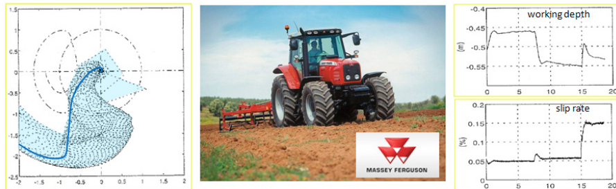
FIGURE 4. Robust design of an open-loop Nyquist locus for the control of working depth and slip rate related to a tractor three point hitch
